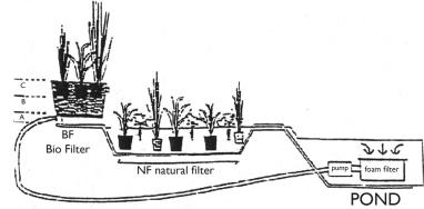
The diagram illustrates the elements integrated into a complete filtration system. Biot-filter sections are:
